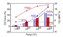
Oxygen-enhanced water gas shift (OWGS) can lead to much higher CO conversion and higher  $H_2$  yield than the conventional water gas shift (WGS) over the same bimetallic Pt–Cu/CeO $_2$  catalyst under comparable reaction conditions.
