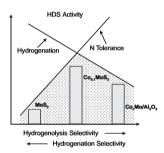
An ultra-deep diesel hydrodesulfurization catalyst such as the unsupported  $Co_{0.1}MoS_2$  requires a balance between the hydrogenation function and resilience to organonitrogen inhibition. The  $Al_2O_3$ -supported  $Co_zMo$  catalyst (z > 0.3) is a commercial hydrodesulfurization catalyst.
