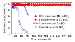
Doping a proper quantity of boric oxide onto a  $Cu-SiO_2$  catalyst significantly improves its stability as well as its activity for the vapor-phase hydrogenation of dimethyl oxalate to ethylene glycol.
