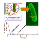
The proposed bactericidal method utilizes *in situ* photoelectrocatalytically generated bactericides to achieve instant inactivation and rapid decomposition of Gram-negative bacteria. The method is capable of inactivating 99.90% of *Escherichia coli* within 0.4 s and mineralizing over 40% biomass within 600 s.
