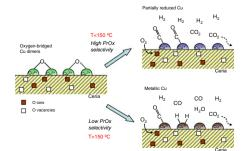
The origin of preferential oxidation (PROX) of CO in the presence of  $H_2$  was traced to the carbonyl stabilization on partially-reduced copper oxide surface, at below 150 °C, preventing thus incoming  $H_2$  from approaching the oxidation sites.
